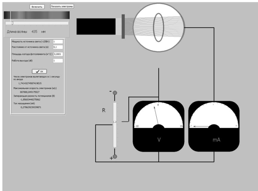
Figure 1. Laboratory work interface of “External photoelectric effect”
